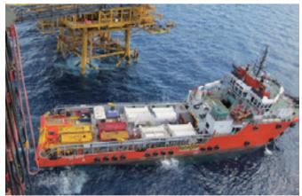
A supply vessel provides CO<sub>2</sub> for injection into the reservoir.
