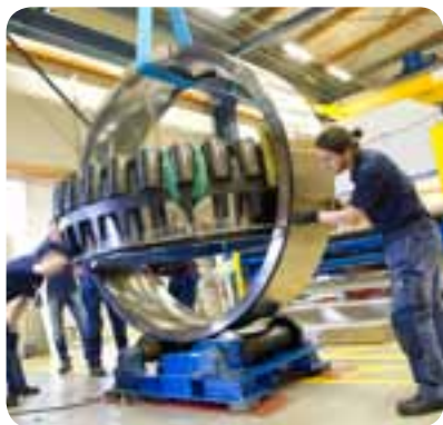
SKF's factory in Gothenburg manufactured two custom-designed spherical roller bearings for the world's largest observation wheel – the Las Vegas High Roller.
