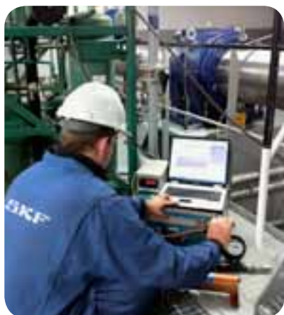
SKF Marine service engineer performing shaft jack up test.
