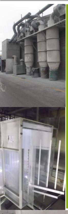
electrostatic We use painting process, we set up a pair of extractors to contain and control air emissions, To harness the process we created a system for the air that is used to remove the paint, either cleaned or injected again into the plant, having benefit as lowering down the high temperature in the summer time within the plant.
