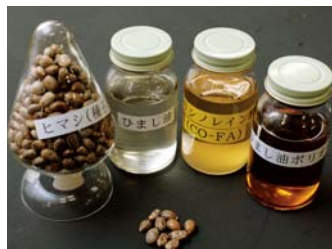
On the far left are castor seeds used as a raw material. To the right, castor oil is processed and refined into ricinoleic acid, which is used to make castor-oil polyol, shown on the far right.
