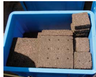
Foundation bed using Mitsui Chemicals' diphenylmethane diisocyanate (MDI)
