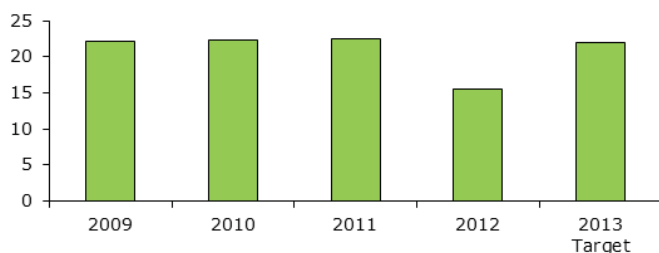
Dry matter in waste water for every ton product produced at our chocolate factory (Average of kg dry matter/ton product)
