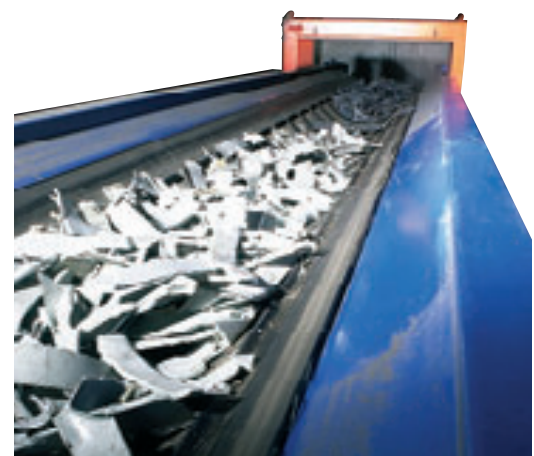
Grinding end-of-life wheeled containers at the Plastic Recycling plant in Saint Eusèbe, France
