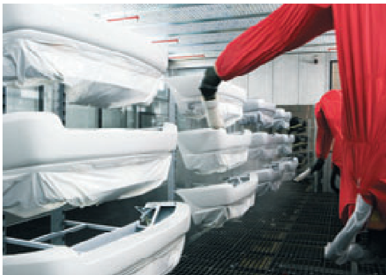
New paint line equipped with a dual system for reducing VOCs, at the Anderson, South Carolina plant
