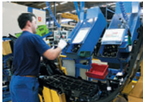
Assembly workstation that can be adjusted vertically to the operator's height
