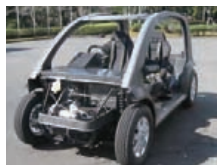
Structure of concept car made entirely of thermoplastic CFRP
