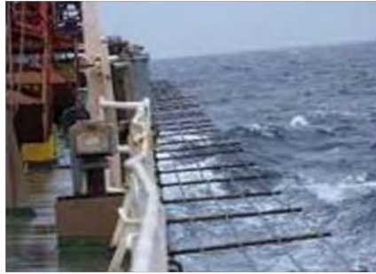
(Wire web installed on the ship to prevent boarding of pirates)
