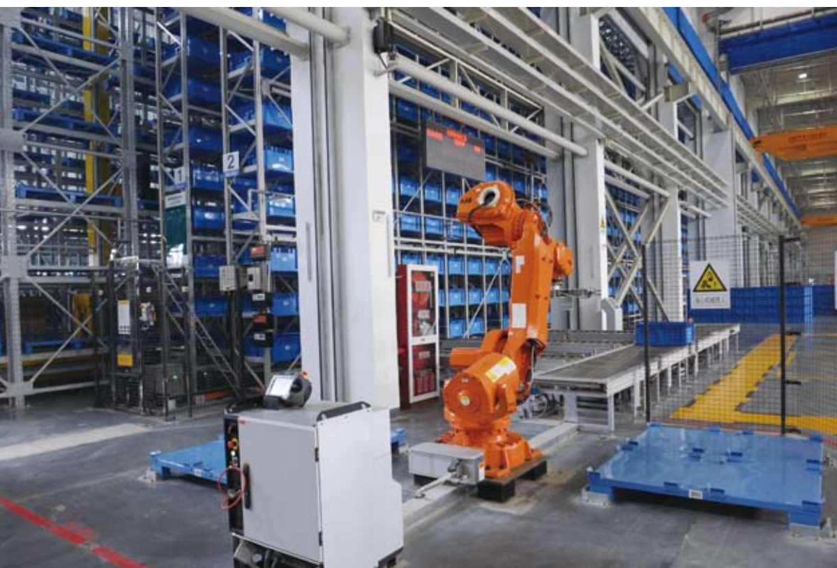
Nanjing Center Warehouse of Jiangsu Electric Power Company realized the intellectualization of the whole storage and delivery process including mechanical shipping, code identification, electrical scanning and automatic packaging
