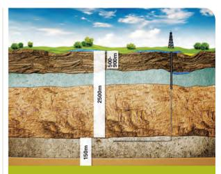
To unlock shale gas, Nexen horizontally drills and stimulates (fractures) gas-bearing zones, most of which are located hundreds or thousands of metres below groundwater aquifers. Multiple layers of cement and protective steel casing in the well provide well control and protection of water sources.
