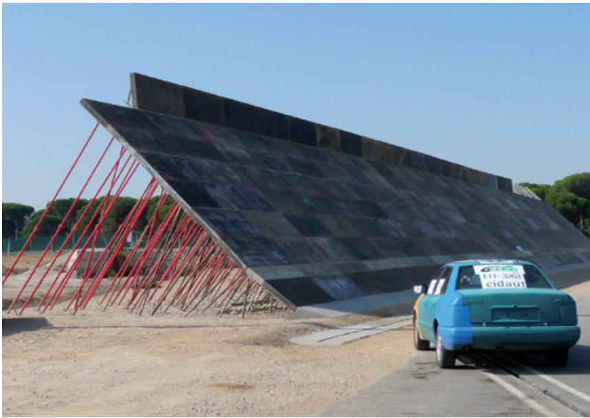
Trials carried out by the OASIS project in barrier-free road banks with side slopes, to increase highway safety.
