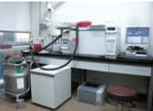
Indoor air quality VoCs tester (GC-MSD)
