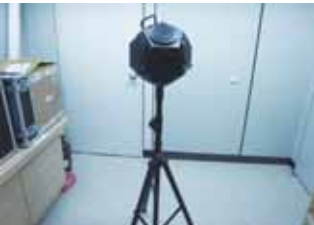
Testing sound between dry-walled rooms (Sound source)
