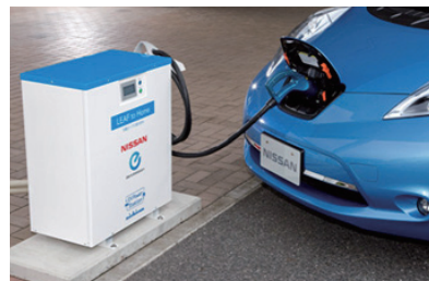
The “LEAF to Home” system in action, using the EV Power Station released by Nichikon in June 2012
