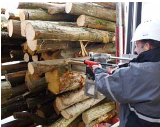
Taking samples for Quality Control during the reception of wood to feed the biomass boiler at Beinheim (France).
