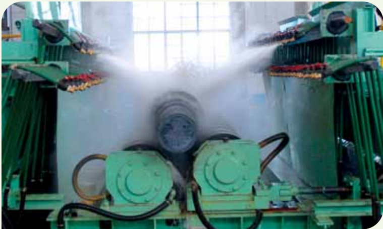
喷淬水系统循环水使用的创新举措，大幅降低了新水采集量。经统计，每年可节约新水 2 万余吨。 The innovative recycled use of quenching water helps significantly reduce new water consumption. According to statistics, over 20,000 tons of water can be saved every year.
