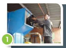
The process begins with crate granulation. The crates are ground into chips, a process which is often performed at our plants or depots, and shipped to the supplier in bags.
