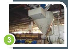
The clean material is drawn from the silos into a pelletiser via a hopper. Additives and Masterbatch are then blended into the mixture, facilitating effective material bonding and colour compliance. The material is then pelletised by melting and chopping it into consistent sized pellets.
