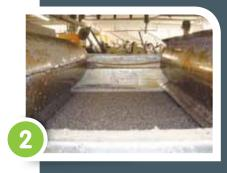
The granulated material is then sent to a washer in order to remove any contaminants such as sand, stones, and dirt. The washed material is dried to remove all water and fluff and then sucked directly into dedicated silos.
