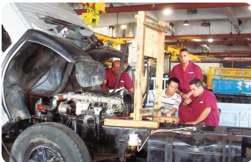
Yuchai technicians are guiding Yuchai Cuba service station staff to installate Yuchai engine
