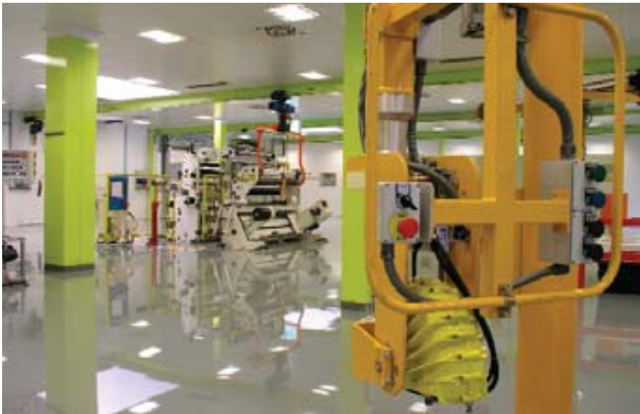
The AP Singen Pharma-Centre (operating in accordance with the ISO 14644-1 regulation, class ISO 8, FED 100.000) carries out reel slitting and pre-packing of flexible primary packing materials for pharmaceutical applications under clean room conditions.
