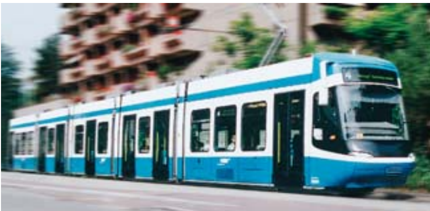
Articulated low-floor tramway named Cobra built by Bombardier Transportation (Switzerland) Ltd for Zurich Transit Authorities using structural aluminum components, sandwich panels and composite driver cabs from Alcan.
