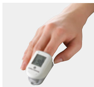
"PULSOX-1" pulse oximeter which measures oxygen saturation in the blood, without the need for blood collection
