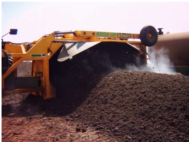
Windrow turner aerating a compost pile and injecting incorporating vinasse
