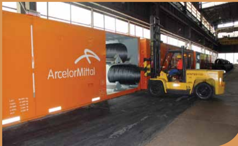
Special machine-thread car developed at Monlevade: guarantee of integrity of cargo
