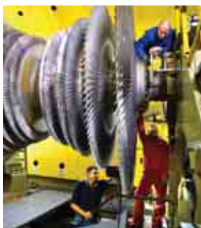
A rotor from Camden power station is being balanced at the Rotek facility
