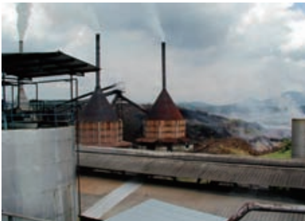
Power generation using coconut shells as fuel
