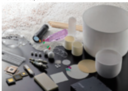
Alumina powder and products made from alumina
