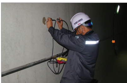
■ Precise inspection for facilities (Measuring the crevice depth)
