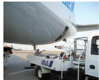
Wastewater operations and wastewater truck
