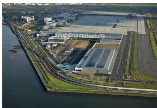
Photovoltaic cells covering the shed of International Cargo Building No. 2
