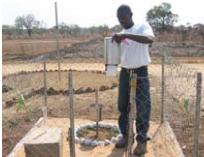
Under the flood-warning system, precipitation levels are measured daily and critical readings reported.
