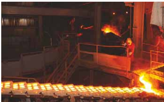
Blast furnace hot metal pouring area at PID, Amona
