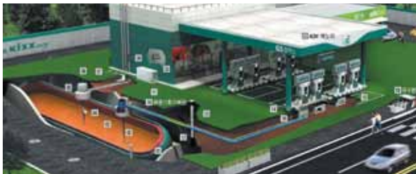
The definition of a clean gas station-Clean gas stations are equipped with proactive systems to prevent soil contamination by double-walled tanks (FRP+iron plates, HDPE), double-walled pipes, equipments to prevent oil leak and overflow and oil leak sensors.
