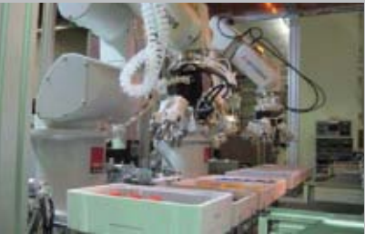
Robot-controlled cell production system equipped with a second-generation hand in operation in our Takino Plant
