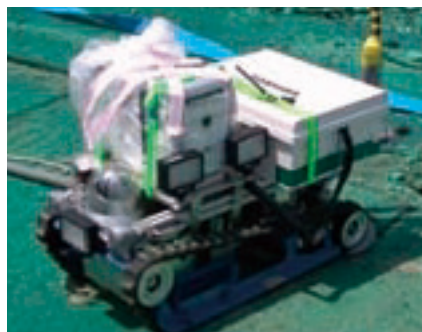
Gamma camera used at the Fukushima Daiichi Nuclear Power Station to measure radiation dose rates
