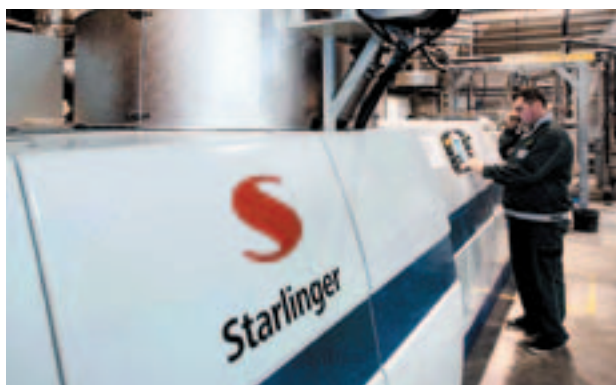
At the Pet-to-Pet Recycling plant in Muellendorf, Austria, a new processing line has been installed. The state-of-the-art recycling plant has been producing PET flakes from recycled PET bottles for many years and now using the latest technologies to turn used PET bottles into granulate.
