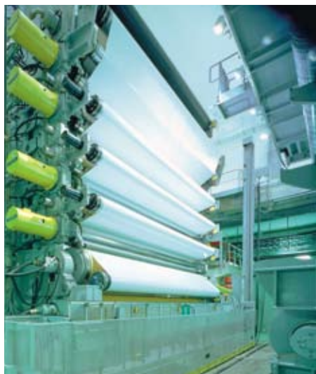
Super calender, Gratkorn Mill, Austria
