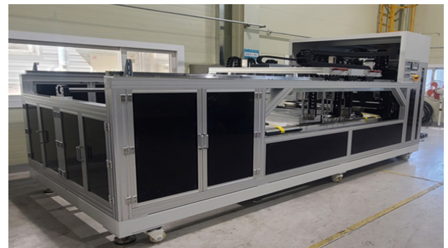
Recycling device of waste photovoltaic modules, glass separator
