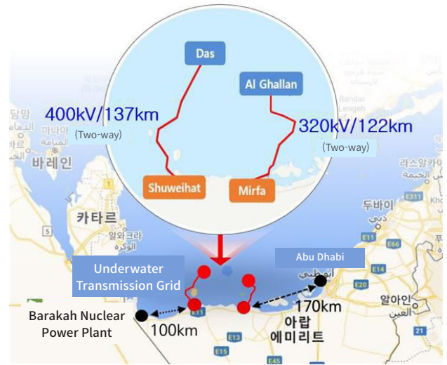
KEPCO | The Conceptual Diagram of UAE HVDC Transmission Grid
