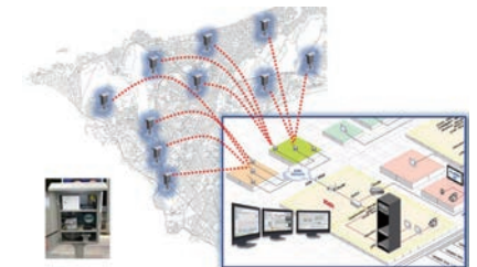
Water supply management system and measuring equipment
