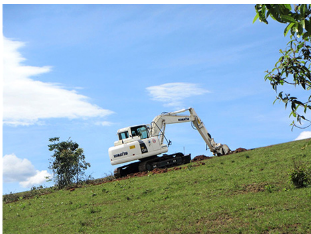
Komatsu's Demining Machine
