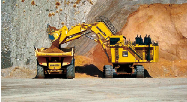
PC7000-11 hydraulic excavator performs loading operations to Innovative Autonomous Haulage Vehicle
