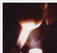
Manufacturing optical fiber preforms using the VAD method
