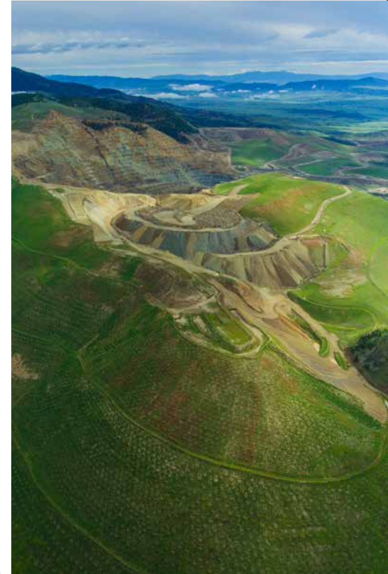
Golden Sunlight mine is reprocessing its tailings and backfilling the open pit - Montana, USA.
