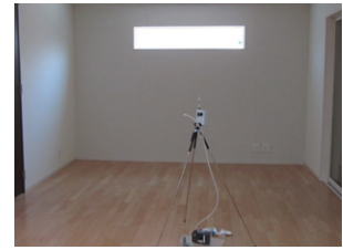
Measuring indoor air quality concentrations
