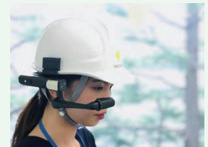
Replacing smart glasses with explosion-proof smart glasses
