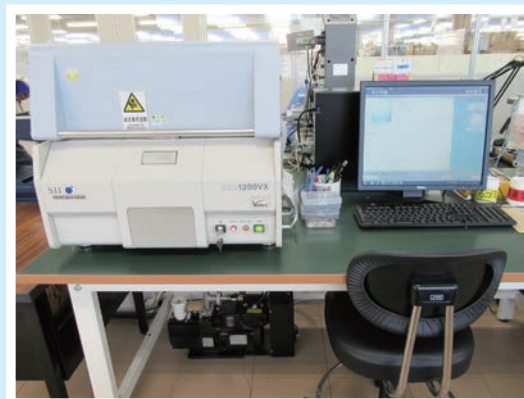
Thermal desorption mass spectrometer (Phthalate ester inspection device)
