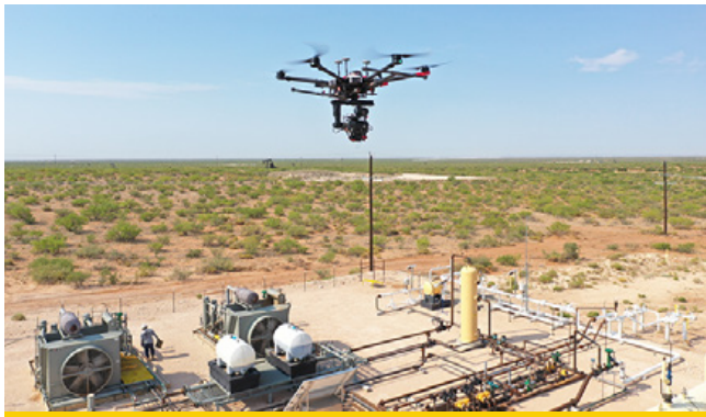
We are expanding our use of drones for methane leak detection at our sites in the Permian Basin, USA.
