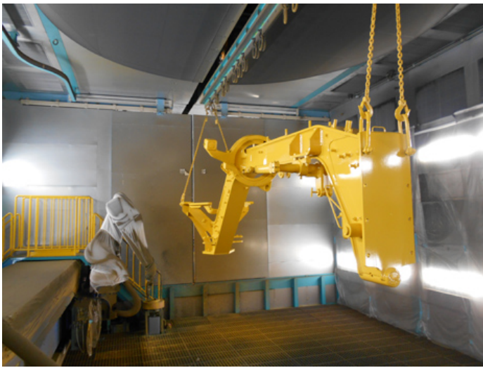
Frame coating with the coating robot
