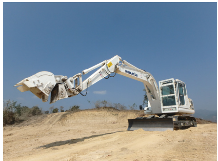
(2) Demining Machine for processing unexploded ordnance
