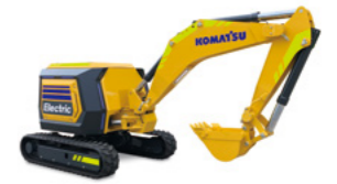
Fully electric and remote-controlled mini excavator concept machine powered by lithium-ion battery
