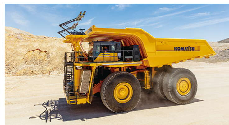
Power agnostic development truck undergoing testing at test site (Arizona, United States)
