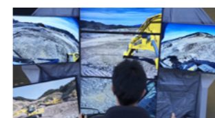
PC200i-11 hydraulic excavator being operated remotely from control pod (Ishikawa Prefecture)
