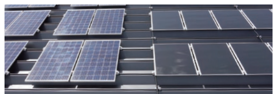
They are placed next to silicon solar cells of another company in order to compare power output.
