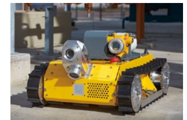
ExRobotics' robot for inspection tasks: ExR-1
