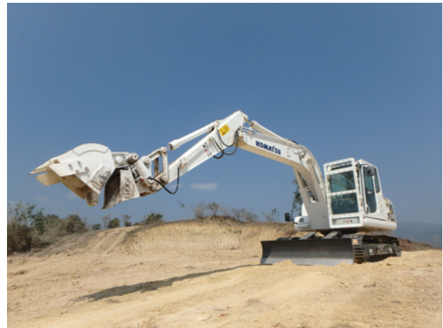
(2) Demining Machine for processing unexploded ordnance
