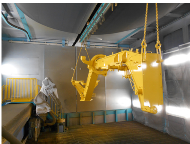
Frame coating with the coating robot
