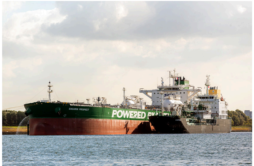
The Cardissa LNG bunker vessel refuels the Gagarin Prospect tanker at the Gate terminal in Rotterdam, the Netherlands.
