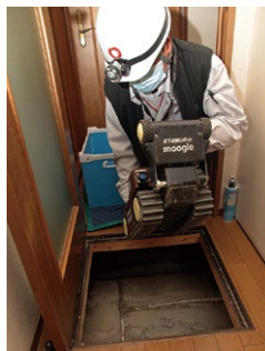
Confined space inspection robot "Moogle"
